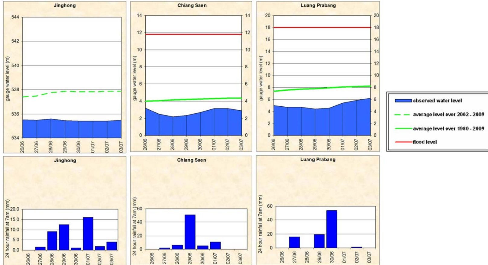
Figure A1: Observed water level and rainfall for Jinghong, Chiang Saen, and Luang Prabang
